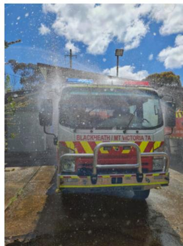
Pictured here is Blackheath/Mount Victoria's Cat 7 tanker testing the cabin protection system during a recent training session. During the fires the Cat 1 tanker was caught in an overrun at a property
